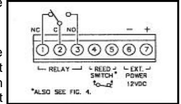
**Relay (Terminals 1-3).** Terminal 1 = Normally Closed; Terminal 2 = Common; Terminal 3 = Normally Open.
